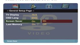
Last Memory—If you turn off your TV with a disc in the disc slot or eject a disc when Last Memory is turned on, then turn on your TV or insert the same disc, playback resumes where it stopped. You can select On or Off.
